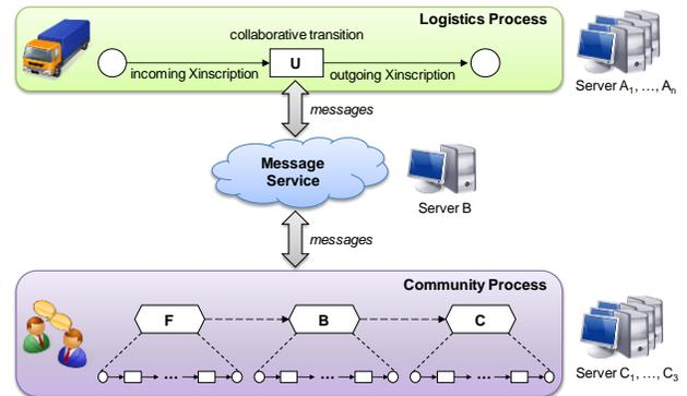
**Figure 2. Concept of the integrated approach**
