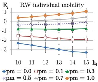
Fig. 2. Error in communication hops when adding mobility
