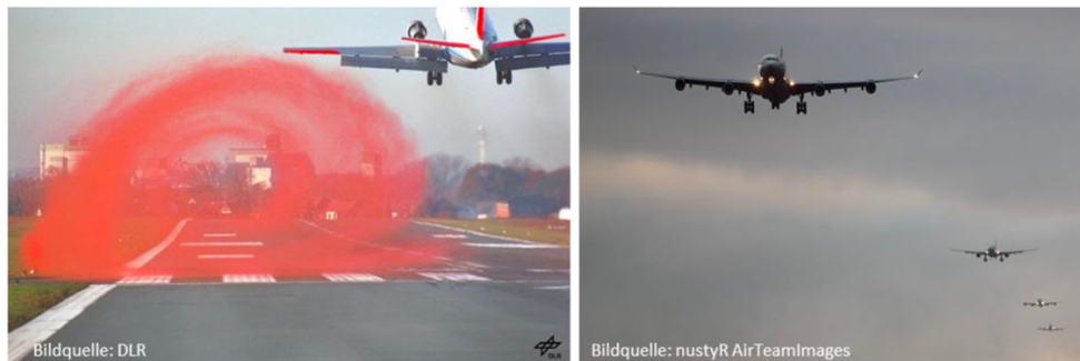
Figure 1: The wake vortex generated by an aircraft during landing (left); aircrafts waiting to land while maintaining a safe distance (right).
