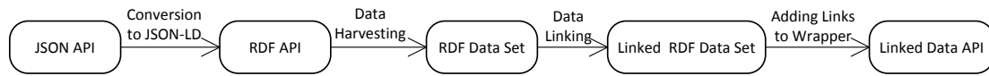
Fig. 1. Schematic view of the steps taken to create a Linked Data version of the CrunchBase API.
